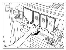
Pull out the seal in the direction of the arrow as shown on the right.
